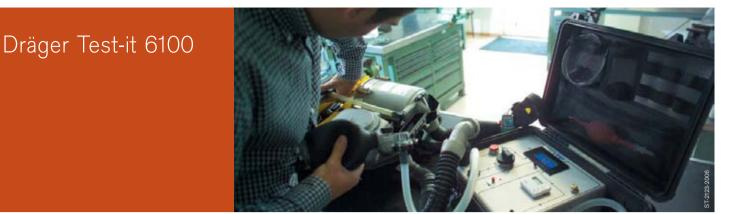
The new Dräger Test-it 6100 is a handy mobile test device designed especially for testing your closed-circuit breathing apparatus. The compact suitcase design includes all the necessary accessories, such as adapters and hoses for the Dräger PSS<sup>®</sup> BG4; offering dependable quality at a low purchase price combined with low operating costs.
